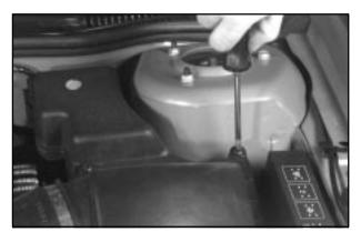
To check or replace the filter, remove the screws that hold the cover on and lift the cover. Be sure to reinstall the air cleaner filter and replace the cover tightly.
